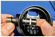
19. Spin on the Heat Exchanger (1) finger tight.
