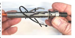
16. Using a fingernail, remove the LP seat (16) from the Poppet (17). With a thin pick, carefully remove the inner o-ring (18) before the outer o-ring (19). Set the component parts aside.
