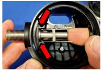
18. Add o-ring (2) to the threaded end of the barrel.
