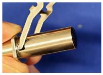
16. Insert the barrel into the case through the larger hole with the notch. Control the lever so that it does not spring up when it clears the inside of the case.
