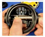
11. Rotate the barrel 90 degrees, and keeping the lever flat against the barrel, slide it out of the case.
